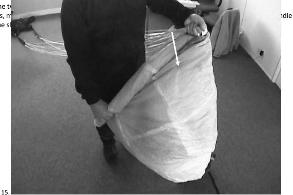
Gently swing the canopy out and lay it on the floor as shown. Carefully push the air out of the canopy. Again, make sure that the slider stays in place against the slider stops. WARNING: IF THE SLIDER IS NOT AGAINST THE SLIDER STOPS, THE POSSIBILITY OF A HARD OPENING AND SERIOUS INJURY OR DEATH IS SIGNIFICANTLY INCREASED.
